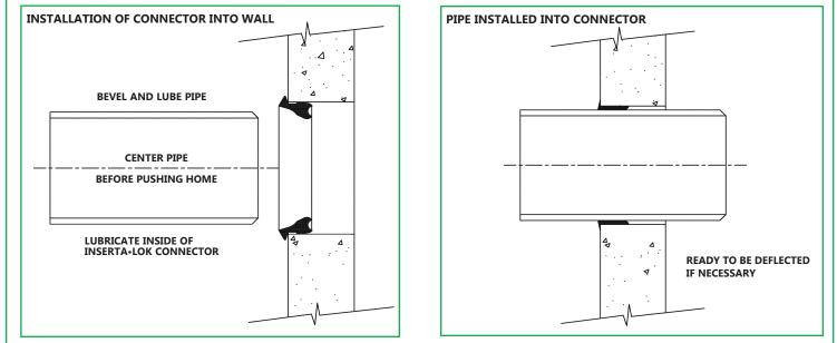
**WARNING:** To ensure the INSERTA•LOK<sup>™</sup> Connector remains a flexible, watertight joint, it is A•LOK Products, Inc. strong recommendation that <u>no mortar</u> be placed between the pipe and wall of the precast concrete unit. The use of mortar in this area would eliminate the flexibility for which the connector was designed and cause problems of shear.
