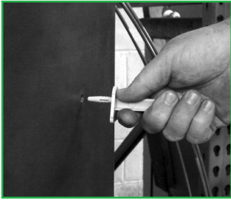
STEP 1: Align locking mechanism into drilled hole.
