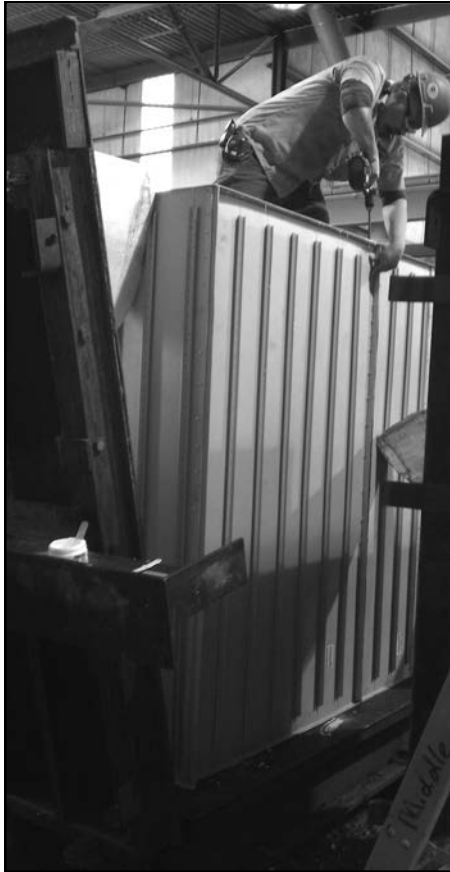
Figure 3 - Duraplate Liner attached to box bottom
