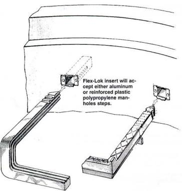
Since the insert is made of polypropylene, It has a life expectancy which exceeds the concrete itself, and has excellent chemical resistance.
