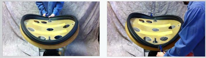
Place two grips at 12 & 6 o'clock (the two lowest points on a curved mandrel) with the clamps underneath the outside half of the mandrel. Pull the clamp trigger until the 2 hooks fit snugly into the waterstop of the connector and starts pulling the connector down (see picture below).
