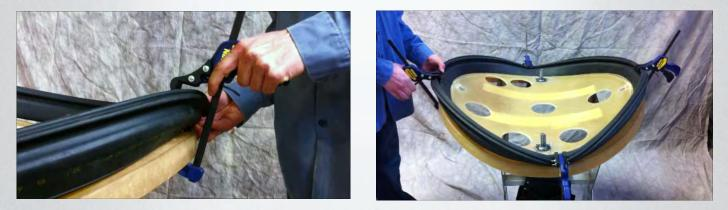
Position the other two clamps at 3 and 9 o'clock. Once all four clamps are installed, make sure the nose of the connector is consistently tight against the offset.
