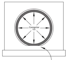
Note: Mandrels size 600 and above - Flat spot must be placed on the outside towards the bottom of the structure to ensure pipe will be centered in connector during installation.
