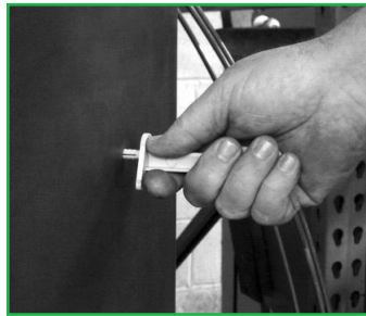
STEP 2: Insert locking mechanism into drilled hole.
